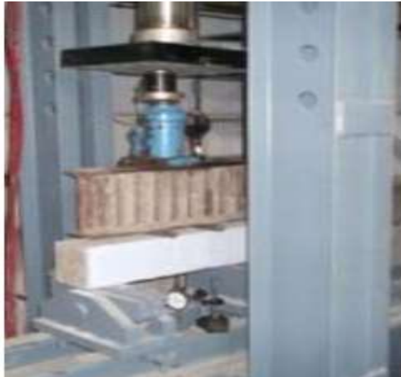
Figure 4: Experimental setup for two point flexural loading
