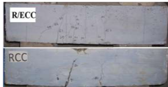
Figure 6: Crack pattern of R/ECC and RCC beams after testing
