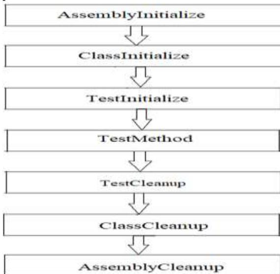
**Fig3:Attributes used in test execution in Coded UI Framework**
