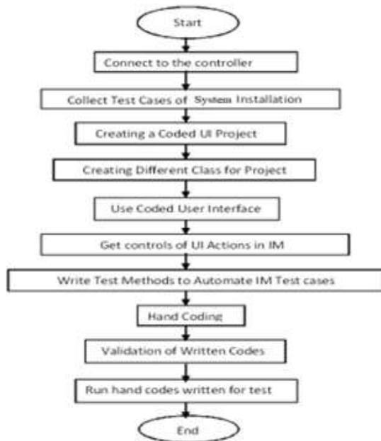
Fig1:Steps used to execute automation test cases. Fig 1 clarifies about the hand coding on computerization test cases PC is associated with a controller and gather the experiments of Related to the establishment supervisor, make a coded UI venture and particular class at that point utilize the coded UI to interface all the task and get controls on
