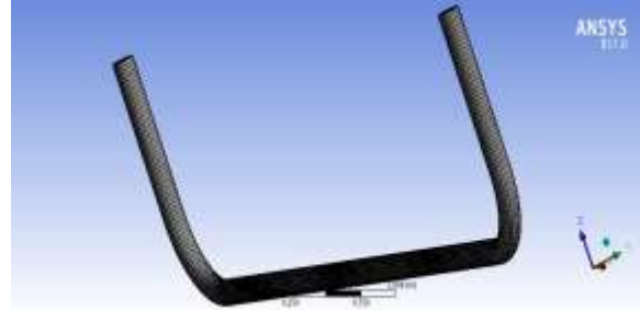
Figure 3 Meshing of earth air heat exchanger without fin for PVC and Aluminium.
