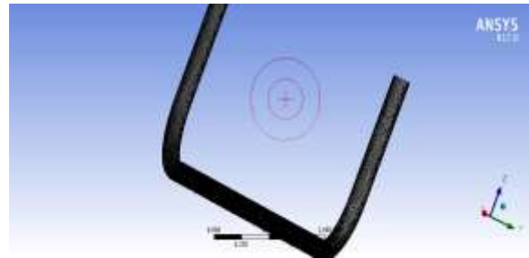
Figure 4 Meshing of earth air heat exchanger with fin for PVC and Aluminium.
