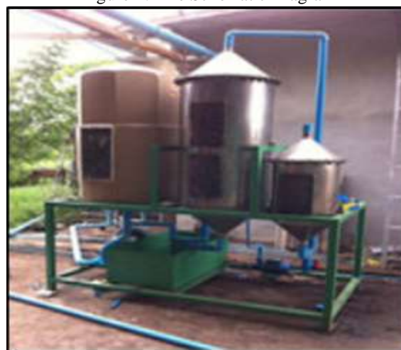
Figure 2: The Purification Biogas System
