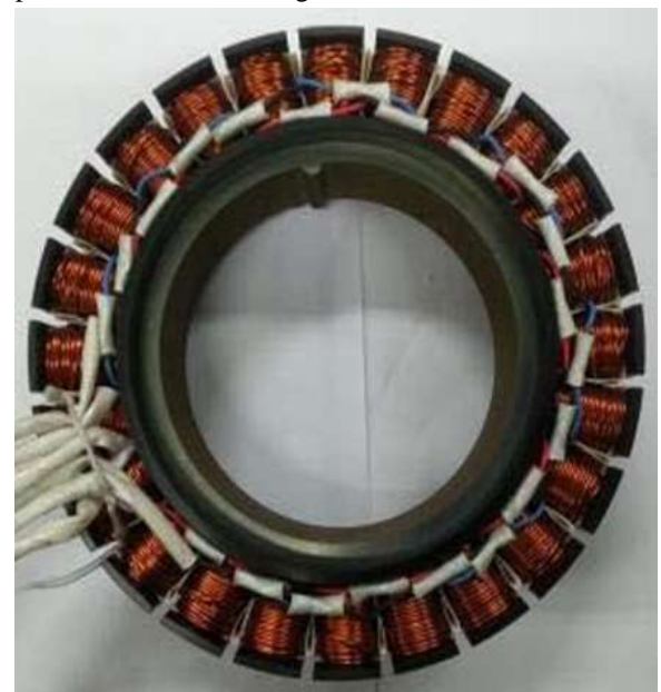
Fig. 2. Prototype of the miniature model (16 poles and 24 slots).
