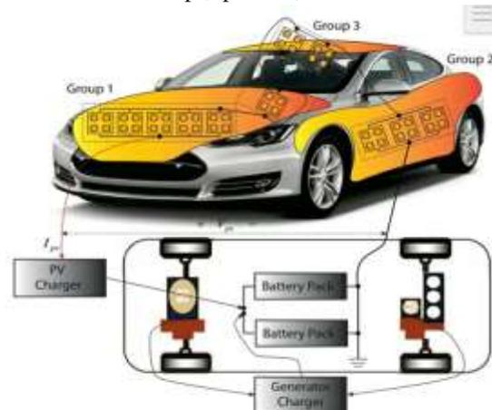
Fig. 4. System diagram of an LSC-based PV system on an HPEV.
