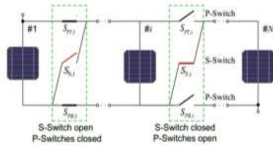
Fig. 3. The structure of a reconfigurable PV array.
