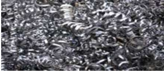
Fig (3.2): metal scraps produced from machining processes, used for making outer surface grid
