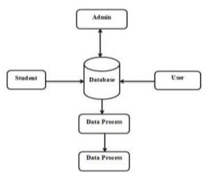
In these system there are three modules Administrator module, Student module and User module, all can access the data and services. The Admin module has special authority. Admin is host of the system which will update and delete data whenever necessary. Student module is designed which has login through which they can access the services of site. Through user module user can only take virtual view of website.
