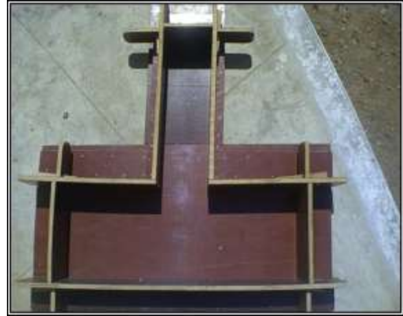
Fig 4 Formwork for casting the specimens
