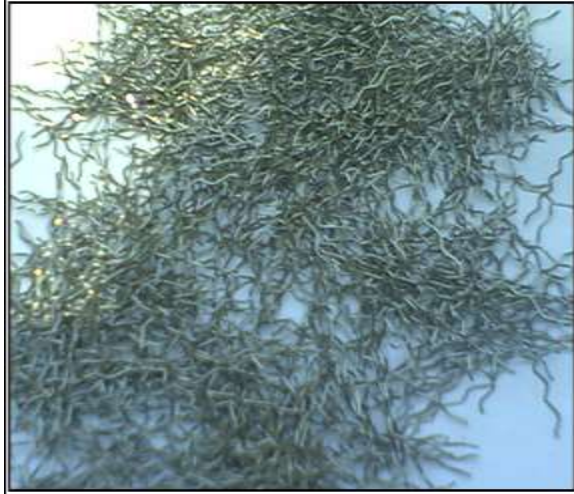
Fig 3 Round and Crimped Steel Fibres
