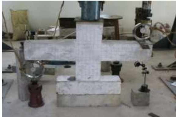
Fig 6 Experimental setup SFRC Beam-Column joint
