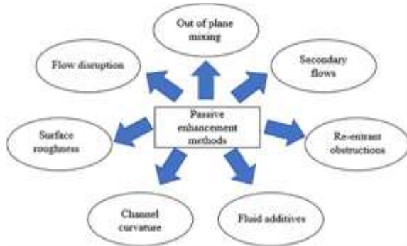
Figure 1 Passive Techniques for Heat Transfer Augmentation
