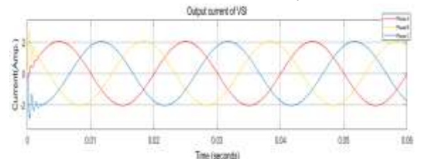
Fig.4.10 Output current of VSI using third harmonic injection PWM at carrier frequency ( f_c ) = 8 KHz
