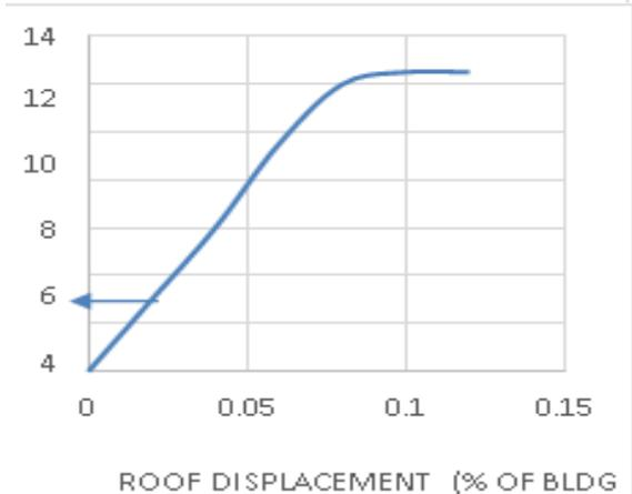
From the pushover curve obtained for the building, we can see that the building has been designed to resist a base shear of 1125.1 kN, but actually it is capable of taking upto about 3500Kn
