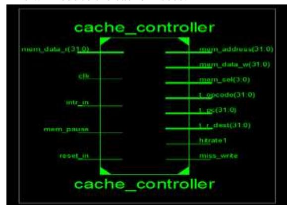
Fig3: RTL view of Cache Controller
