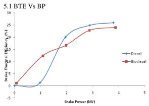
Graph shows variation in brake thermal efficiency for different fuels. Lower brake thermal efficiency is observed with cotton seed bio diesel due to its higher viscosity and low volatility. Due to higher viscosity, injection of larger droplets causes slow evaporation, poor air- fuel mixing and slow combustion which results in lower thermal efficiency.
