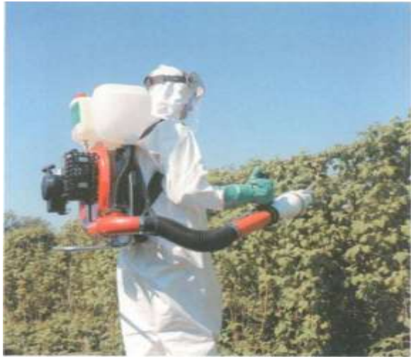
Fig 1.2 Engine operated sprayer
