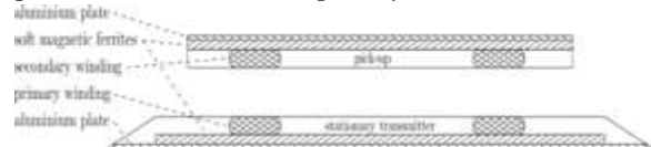
Figure 2: Schematic diagram of the inductive system's cross section
