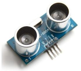
Fig 4.7) Ultrasonic Sensor Ultrasonic sensors are a type of acoustic sensor. This contains one transmitter and one receiver. Transmitters convert electrical signals into ultrasound receivers convert ultrasound into electrical signals. In similar way radar and sonar, ultrasonic sensors are used in systems which evaluate targets by interpreting the reflected signals. For example, by measuring the time between sending a signal and receiving an echo the distance of an object can be calculated.
