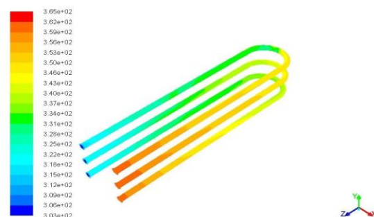
Fig.5 Contours of Static temperature on U- tube
