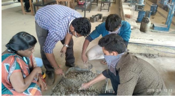
Figure 5-Mixing of Fly ash with Alkaline Solutions For instance, NaOH solution with a concentration of 16 Molar consists of 16 \times 40 = 640 grams of NaOH solids per litre of the water, where 40 is the molecular weight of NaOH. Note that the mass of water is the major component in both the alkaline solutions. The mass of NaOH solids was measured as 444 grams per kg of NaOH solution with a Concentration of 16 Molar. Similarly, the mass of NaOH solids per kg of the solution for other concentrations was measured as 10 Molar: 314 grams, 12 Molar: 361 grams, and 14 Molar: 404 grams.
