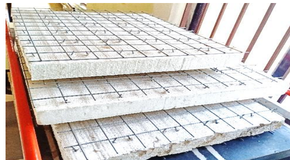
Figure 4-Layers of Welded Mesh infilled with EPS
