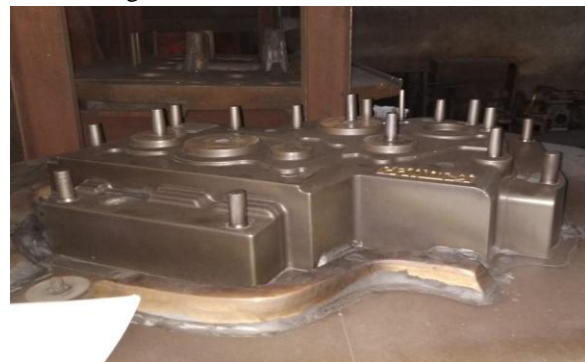
Figure No. 3 Casting with gating system.
