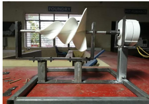
Fig 3 - Fabricated turbine assembly
