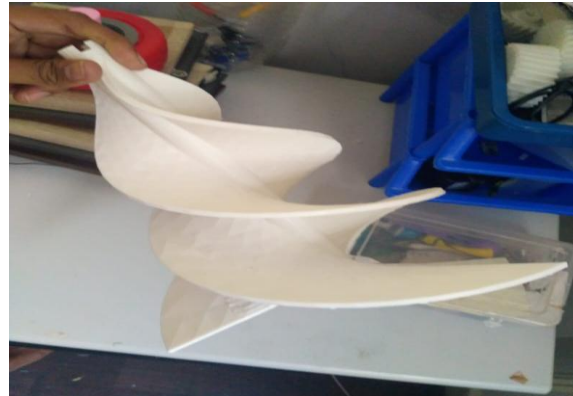
Fig 2 - 3D Printed blade
