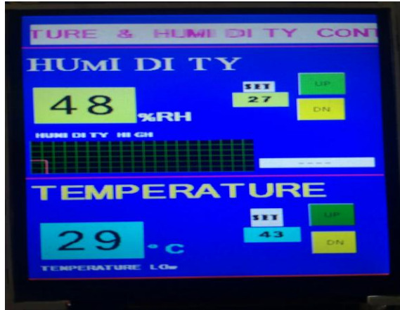
Fig-5 Display of temperature below set point and humidity above set point.
