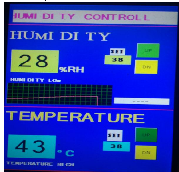
Fig- 4 Display of temperature above set point and humidity below set point.
