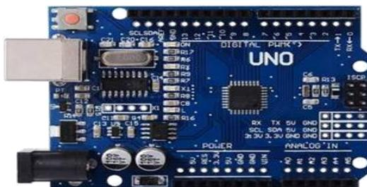
The output of the comparator is given to the digital pin 8. The Arduino is programmed in such a way that whenever there is an input high at the digital pin 8, then the TX pin i.e. pin1 gets activated and the transmitter Bluetooth module which is acting as
