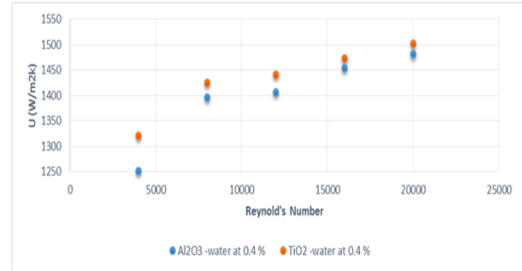
Figure 11 Comparison of overall heat transfer coefficient for different nano fluids at 0.4 % volume fraction
