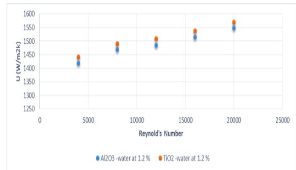
Figure 13 Comparison of overall heat transfer coefficient for different nano fluids at 1.2 % volume fraction
