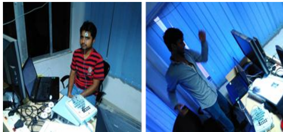
(a) Resting ECG recording with sitting position (b) Extensive activity condition with standing position Fig. 8. Experimental set-up for recording the ECG signals in real time using Allengers Virgo multilead ECG/EEG data acquisition system.
