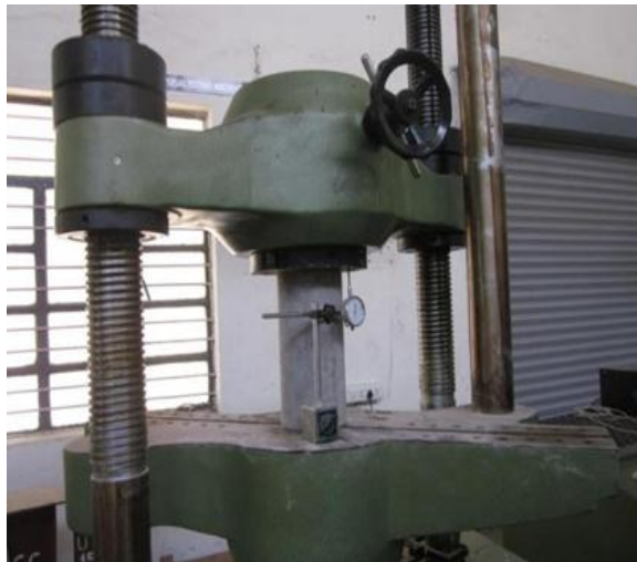
Figure 3 : Testing of Cylindrical Specimen
