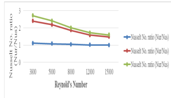
Figure 12 Variation of Nusselt number ratio, Nu_{rib}/Nu_{smooth} with Reynolds number
