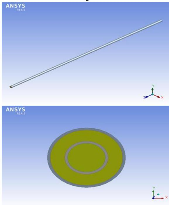
Figure 2 Geometrical model of double pipe heat exchanger.
