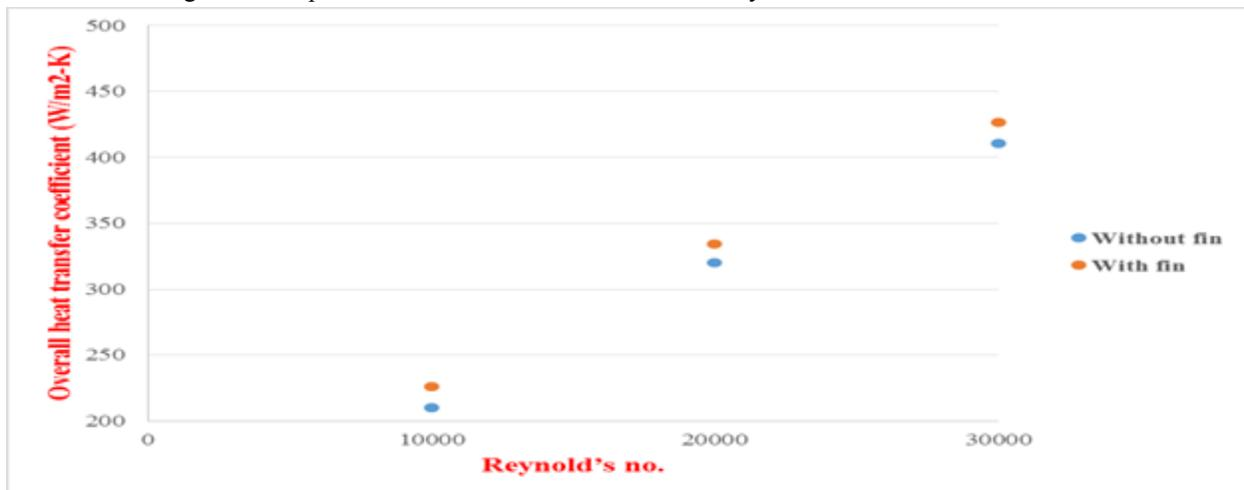
Figure 9 Comparison of Overall heat transfer coefficient at different Reynold's no. with and without fin.
