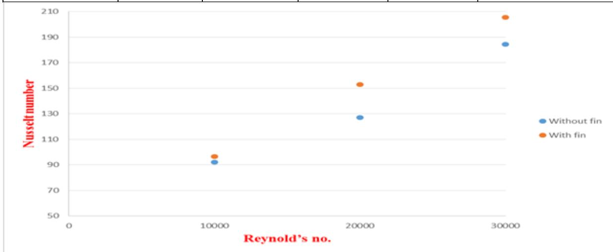
Figure 8 Comparison of Nusselt number at different Reynold's no. with and without fin
