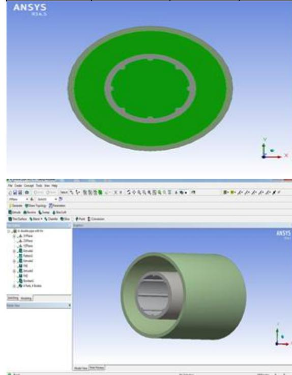
Figure 1 Geometry of double pipe heat exchanger with fin
