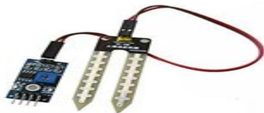
Soil moisture sensors measure the volumetric water content in soil. Since the direct gravimetric measurement of free soil moisture requires removing, drying, and weighting of a sample, soil moisture sensors measure the volumetric water content indirectly by using some other property of the soil, such as electrical resistance, dielectric constant, or interaction with neutrons, as a proxy for the moisture content.
