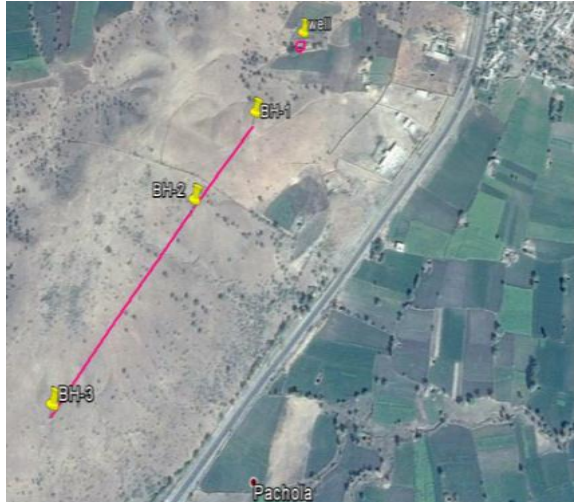
Figure 2 : Tunnel-1 Center line and location of boreholes
