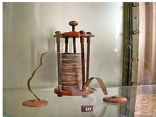
A voltaic pile, the first chemical battery
