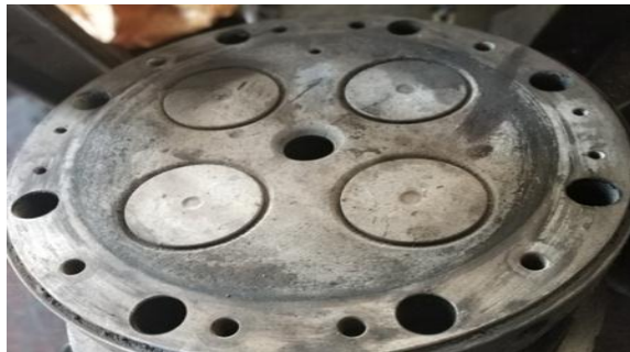
Figure: Valve Seat Wear Due to cyclic loading
