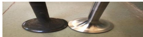
Figure: Failed and New Valve Comparison
