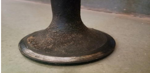
Figure: Valve Face Wear
