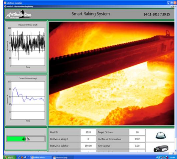
Fig. 11: Picture of the Raking while skimming is going on
