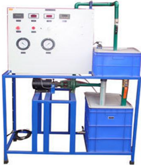
Fig. 1. Experimental set-up of reciprocating pump The following are the steps for the performance testing of a double acting reciprocating pump:
