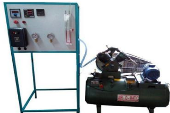
Fig. 1. Experimental set-up of reciprocating air compressor
