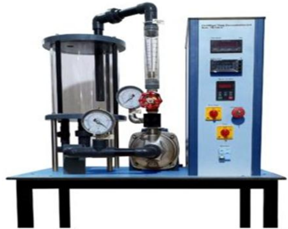
Fig. 1. Experimental set-up of impact of jet The following are the precautions taken while carrying out experiments on impact of jet apparatus.
