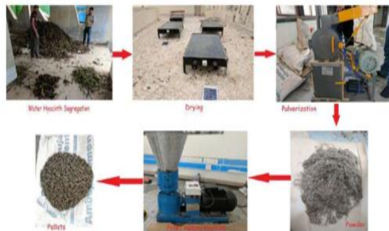
Figure 5: Diagram of fuel pellet manufactures
