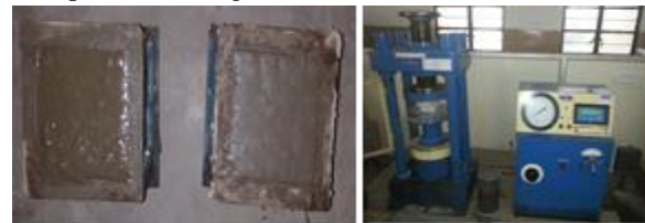
Figure 5: Compressive strength on FAA Concrete
