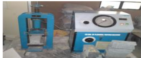
Figure 6: Flexural strength test
