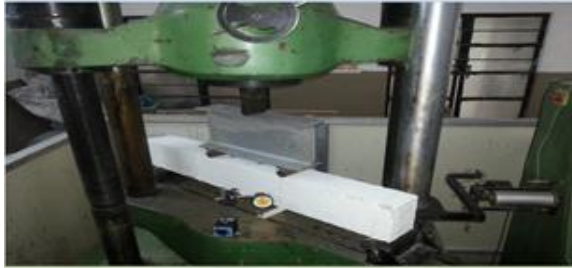
Fig.11. Experimental Setup of the Control RCC Beam
