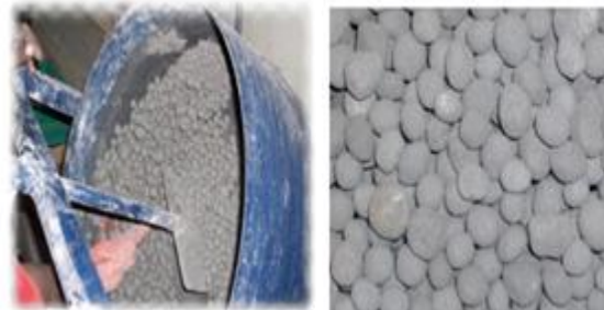
Figure 3: Formation of fly ash Figure 4: Prepared sample of Pellets
