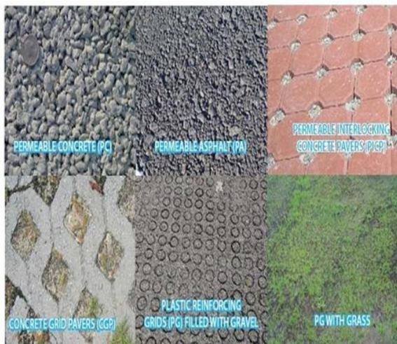
Fig – 1 Types of permeable pavement
