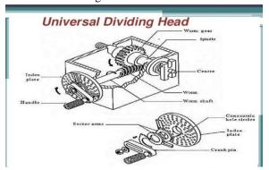
The spindle of the dividing head drivers the work piece. The index plate of a dividing head consists of a no. of holes with a crank and pin. The Index Crank Drivers The Spindle and the live Centre through a Warm Gear Which has generally has 40 teeth full rotation of the work piece is produced by 40 full revolutions of the index crank.
