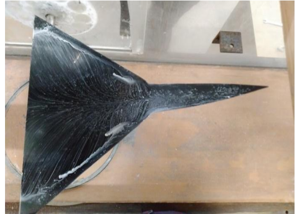
Figure 10: Flow at 30° angle of attack.
