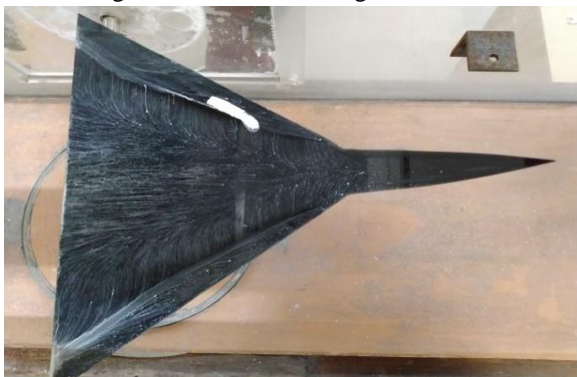
Figure 8: Flow at 15° angle of attack.
