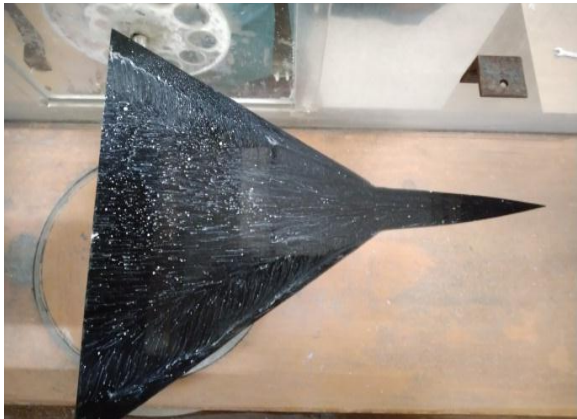
Figure 6: Flow at 5° angle of attack.
