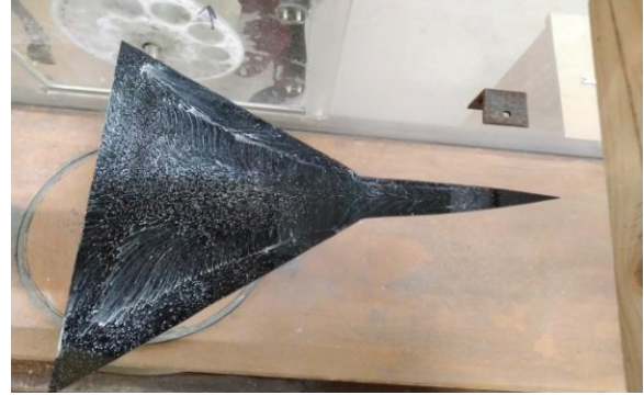
Figure 9: Flow at 20° angle of attack.
