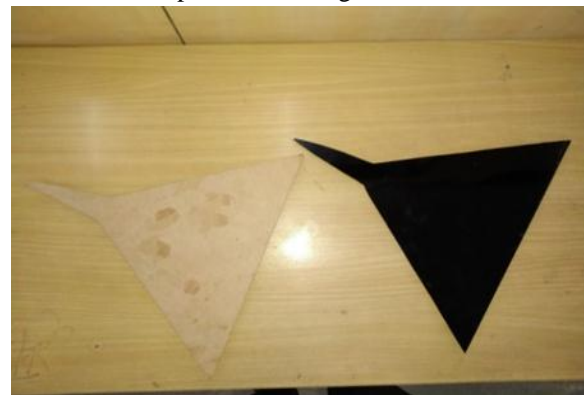
Figure 4: Image of 80/56.867-deg Double-Delta wing.
