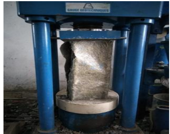
Figure 6: Failure of Double Layered CSM-GFRP Wrapped Column
