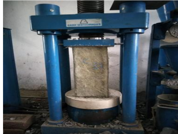
Figure 4: Single Layered CSM-GFRP Wrapped Column Setup
