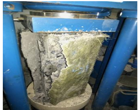
Figure 5: Failure of Single Layered CSM-GFRP Wrapped Column
