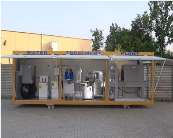
Plate 6: Prefabricated modular water treatment plant
