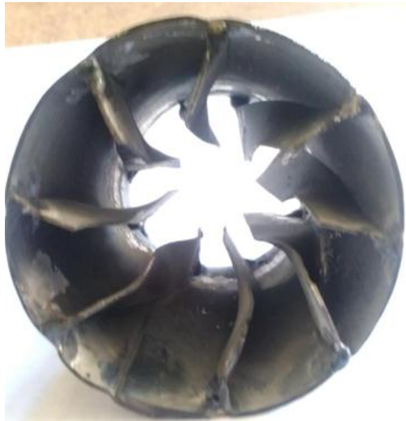
Fig Front view of the conical swirl generator
