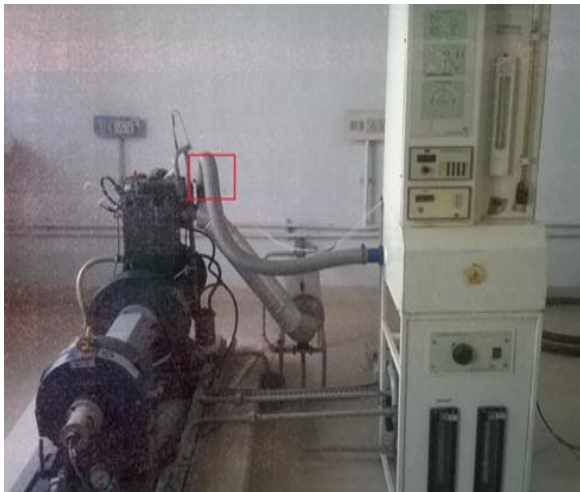
Fig 3.1 Four stroke 1-cylinder diesel engine Experimental test rig with computer interface
