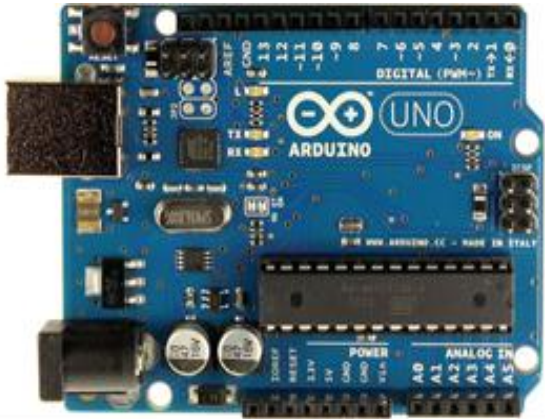
Fig.3 Arduino UNO microcontroller board Arduino UNO is a very basic board in Arduino family which uses Atmega 328P microcontroller. Arduino is an open source embedded system which can be easily programmed as per the required application. Arduino IDE is the required software for programming in Arduino board. Here Arduino is used to program for baby movement and baby cry sensing with the help of PIR and sound sensor.
