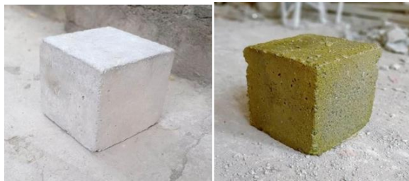
Fig 5.13 Normal cube Fig5.14 Acid affected cube
