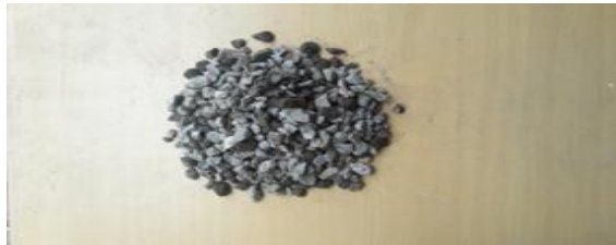
Fig.No.4. 10 mm size recycled aggregate
