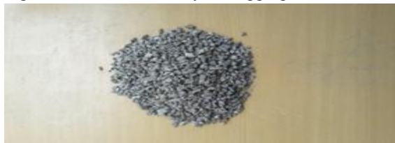
Fig.No.5. 5.6 mm size recycled aggregate
