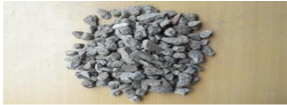
Fig.No.3. 20 mm size recycled aggregate
