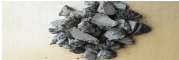
Fig.No.2. 40 mm size recycled aggregate
