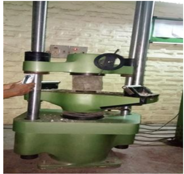
Fig no.7. Testing of a cube on UTM
