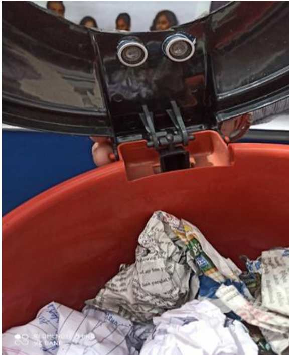
Fig 4. UltraSonic sensor attached to dustbin
