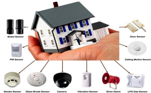
Fig: Components of home security systems
